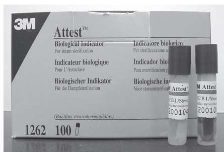
Figure 10.2 Strips containing B. stearothermophilus endospores are placed in the autoclave with the material to be sterilized. After the autoclave cycle is completed, each strip is placed into a broth medium and incubated at 56°C. A second, control strip that has not been autoclaved is incubated in broth at the same time. The endospores on the control strip (left) have germinated, and the growing vegetative cells have made the broth turbid and changed the color of the pH indicator in the broth. The autoclaved endospores (right) have been successfully sterilized and, therefore, the broth remains clear and the original color. ©Josephine A. Morello
