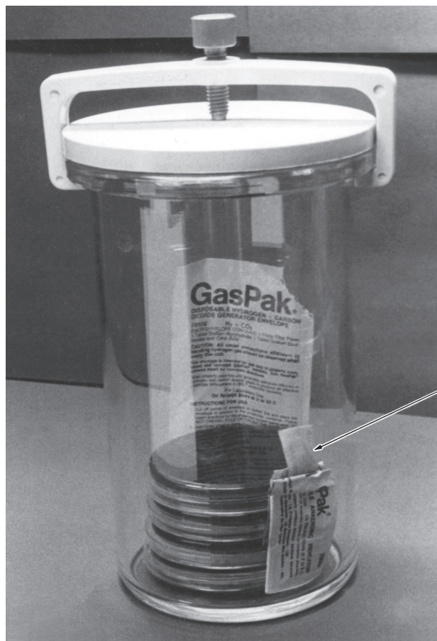
Figure 28.1 A GasPak jar (BD Diagnostic Systems) for cultures to be incubated anaerobically. In this model, the tight-fitting lid contains a catalyst. The large foil envelope has been opened to receive 10 ml of water delivered by a pipette. With the lid clamped in place, hydrogen generated from substances in the large envelope combines with oxygen in the jar’s atmosphere. This combination is mediated by the catalyst and forms water, which condenses on the sides of the jar. Carbon dioxide is also given off by the substances within the large envelope, contributing to the support of growth of fastidious organisms. The smaller envelope has also been opened to expose a pad (arrow) soaked in methylene blue, an indicator used to detect the presence or absence of oxygen. When first exposed, the pad was blue in color. Now it is colorless, indicating that there is no free oxygen left in the jar, for the indicator dye loses its color in the absence of oxygen. The jar now contains an anaerobic atmosphere and can be placed in the incubator. ©Josephine A. Morello
